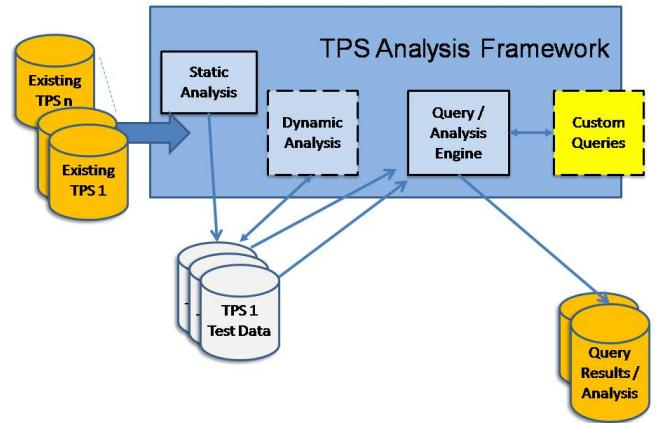
**Figure 1 General architecture for TPS Analysis Framework**
