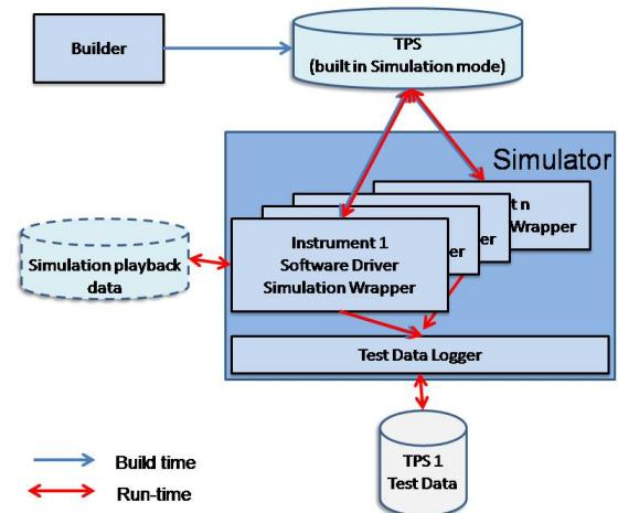
Figure 4 Contents of the Simulator utility in the Framework
